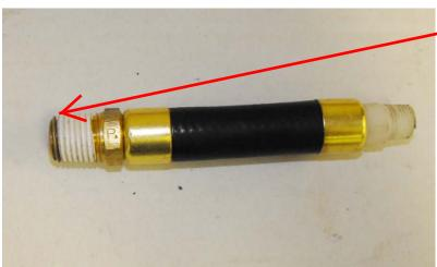
Step # 5 Wrap torch head end of replacement Assembly Coupler Hose with Teflon Tape leave last 2 threads tape free.
