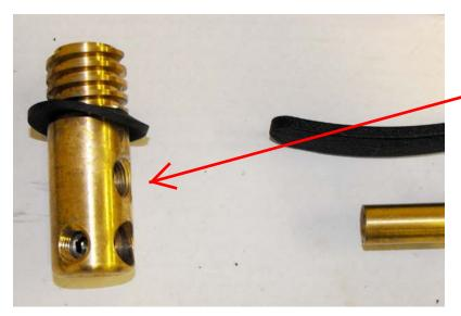
Step # 4 Remove Assembly Coupler Hose from Torch Head
