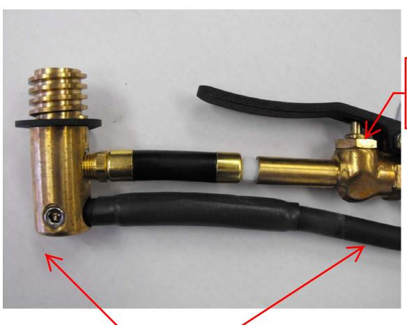
Step # 5 Reinstall valve internals and Valve handle. Pressure and Snoop same. See page # 3
