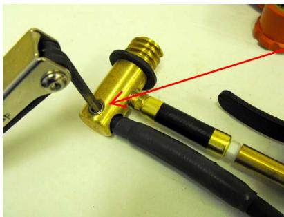
Step # 7 Reinstall Cable into Torch Head and Tighten set screw to Manufactures recommended 20 foot pounds. Snoop as per page # 3
