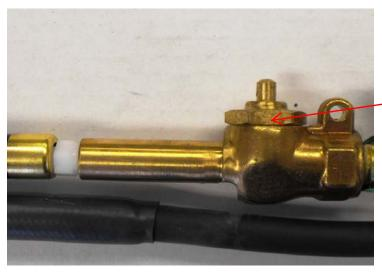
Step # 2 Remove Control valve nut and all internal valve parts
