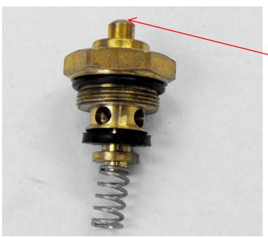
Step # 3 All Internal parts to valve. Brake down to individual parts.
