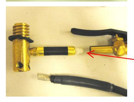
Step # 3 Unscrew Torch Head and Assembly Coupler Hose from Trigger Assembly.
