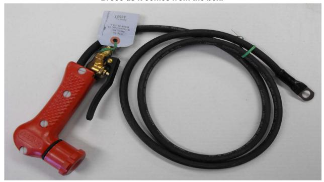
Do not install the torch until you have checked out what is between the handles. This same check out must also be done before every use.
