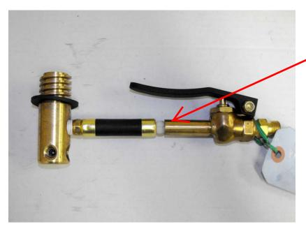
Step # 6 Carefully screw in plastic fitting into trigger assembly. Do not over tighten, or cross thread, you may crack the fitting. There is no Manufacturers recommendation.
