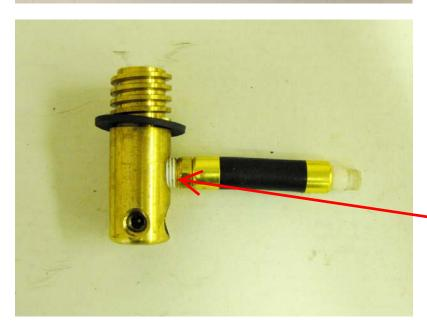
Step # 5 Install Assembly Coupler Hose in Torch Head
