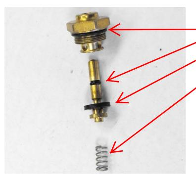
Step # 4 Check both O-rings for damage. replace damaged O-ring.
