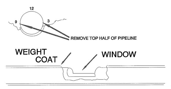
WHEN CUTTING A PIPELINE THAT IS NOT COMPLETELY FREE FROM THE BOTTOM, ALWAYS CLEAR THE COATING FROM THE PIPELINE AND CUT A WINDOW THAT IS AS BIG AS POSSIBLE. THE TOP HALF OF THE PIPELINE IS STRONGLY RECOMMENDED.
