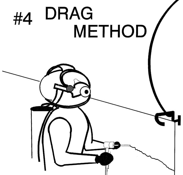
THE DRAG METHOD KEEPS YOUR BODY AND FACE FROM IN FRONT OF THE CUT. YOU PLACE YOUR SELF TO THE SIDE AND DRAG THE ROD TO YOU.
