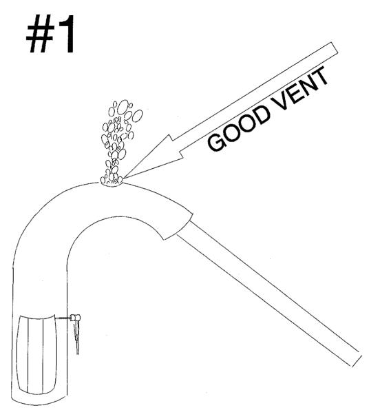
THIS IS A PROPER VENT. NOTE THE VENT IS AT THE HIGHEST POINT WHERE EXPLOSIVE GAS COULD BECOME TRAPPED.
