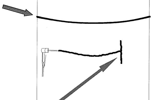
WHEN MAKING A CUT AROUND A PILE OR PIPE WITHOUT A BURNING GUIDE, START WITH A CUT THAT CROSSES THE PLAIN OF YOUR INTENDED BURN. THIS WILL MAKE YOUR TIE IN EASIER
